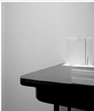
Now rotate the rotator of the Panosaurus (**DO NOT MOVE THE TRIPOD**) until you see the nail and line in the extreme right hand of the frame. The nail and line will **probably** now be out of alignment - either to the right or left of the line. If the nail is to the right of the line this "probably" means the camera needs to be moved further forward on the upper horizontal arm. (This depends on the design of the lens)
