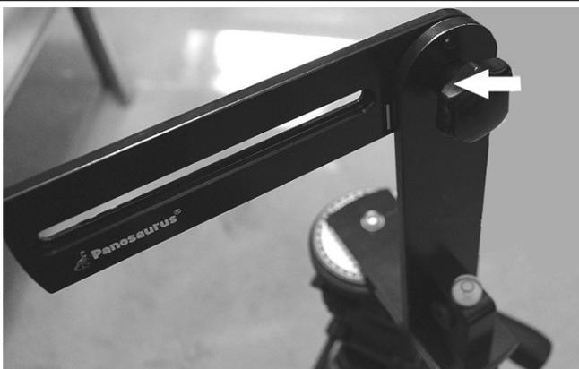
Next - attach the upper horizontal arm to the upright metal arm using the 1/2" bolt clamping knob (**Part 7**).
