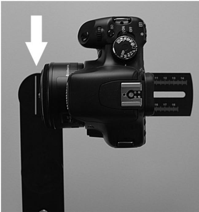
Once your camera is attached to the camera mounting block you will need to check to make sure the camera lens face is parallel to the bold white line at the far end of the upper horizontal arm. To do this slightly loosen the camera mounting block screws and slide the camera on the block down the upper horizontal arm and inspect your alignment.
