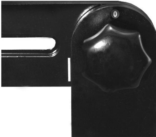
The amount of vertical tilt of the upper horizontal arm is read through the small hole directly above the clamping knob.
