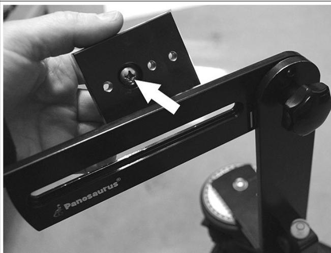
For most cameras and lenses you will attach the camera mounting block to the upper horizontal arm as pictured on the left.
