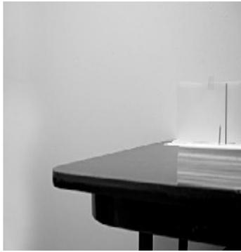
The nail in this picture has moved to the left of the line when it was rotated from the left side of the frame to the right side of the frame. This means that you will probably need to move the camera back toward you on the metal arm. (This depends on the design of the lens)
