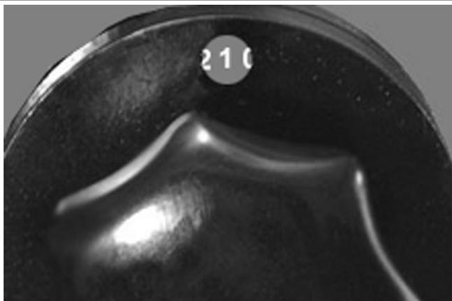
The picture on the left shows 10 degrees of upward vertical tilt - with the 1 mark directly in the center of the hole and equal parts of the 2 and 0 showing on each side of the 1.
