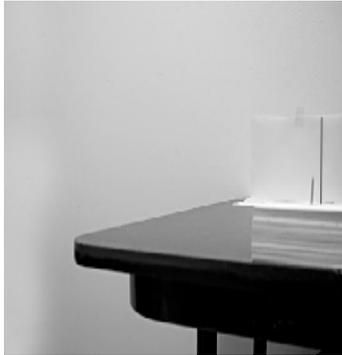
The nail in this picture has moved to the left of the line when it was rotated from the left side of the frame to the right side of the frame. This means that you will probably need to move the camera back toward you on the metal arm.
