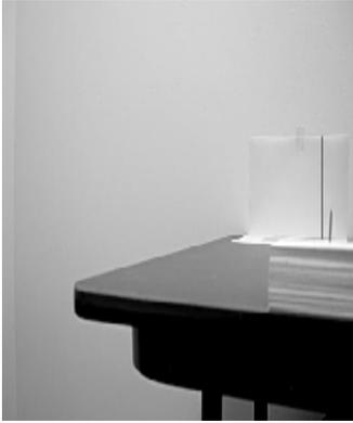
Now rotate the rotator of the Panosaurus (**DO NOT MOVE THE TRIPOD**) until you see the nail and line in the extreme right hand of the frame. The nail and line will **probably** now be out of alignment - either to the right or left of the line. If the nail is to the right of the line this probably means the camera needs to be moved further forward on the metal arm.
