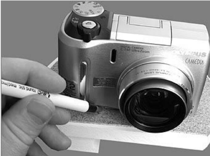
Next, if at all possible, make marks somewhere on the rubber pad, or elsewhere, that will enable you to easily reposition the camera into this same mounting position each time you want to mount the camera to the Mounting Block.
