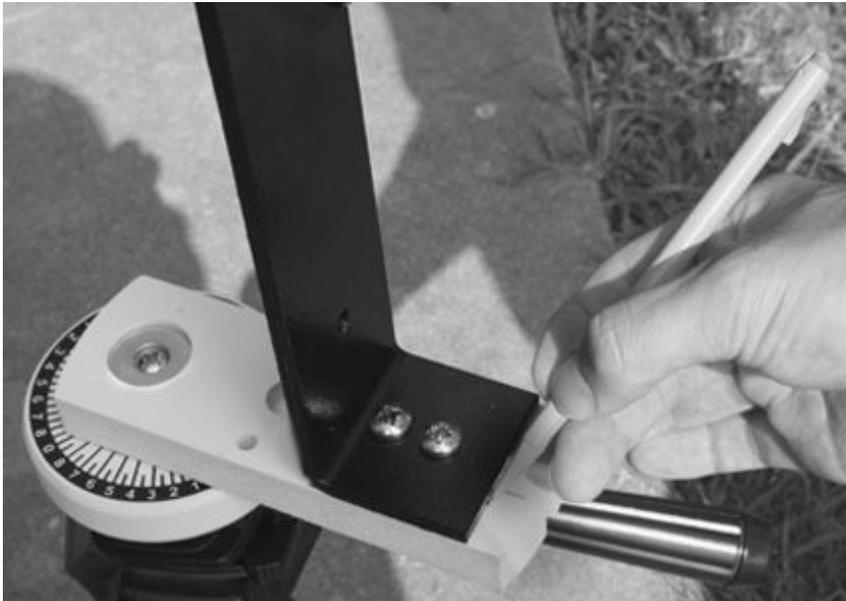
Now make some kind of mark on the Rotator Arm so you will be able to remember exactly where the Metal Arm needs to be placed every time you use this particular camera in the portrait position. You can use a pencil, pen or an sharp edge of some sort to make a permanent mark.
