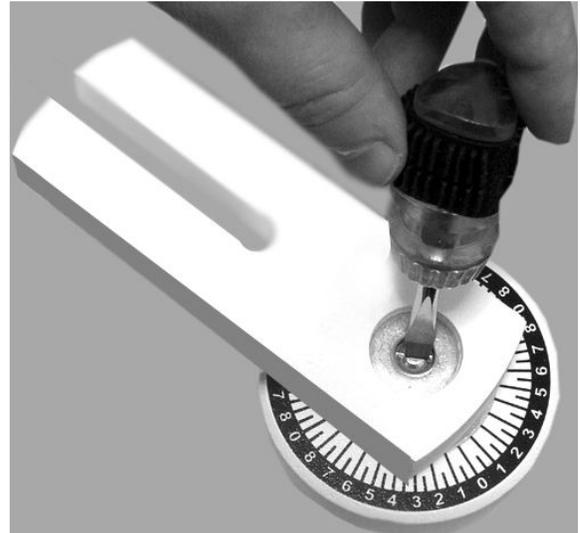
The turntable is laid out in 5 degree increments. There are numbers on the turntable every 10 degrees. You use the extreme front edge of the metal strips screwed to side of the rotator arm (not shown in pictures) to point to the numbers or lines on the turntable. So for example - to shoot a full 360 degree panorama using 9 shots you would shoot your first picture at "0" and then shoot a picture at the numbers 4, 8, 12, 16, 20, 24, 28, and 32.
