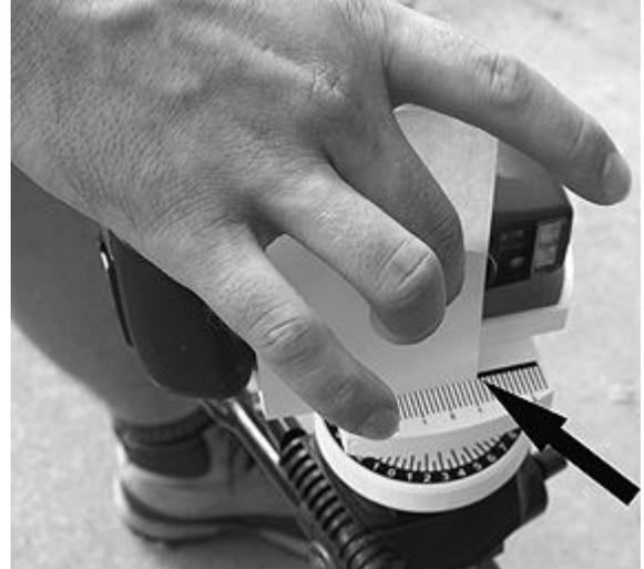
The above pictures show how to use the 3 X 5 index card to help align the lens in the center of the ruled lines. First set the card on the extreme left of the lens and look to see what ruled line touches the bottom of the card. Then do the same thing on the right of the lens. Keep shifting the camera on the rubber pad until the distance from “0” is the same on both the left and right side of the lens barrel.
