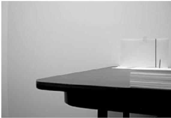
Now rotate the rotator of the Panosaurus (**DO NOT MOVE THE TRIPOD**) until you see the nail and line in the extreme right hand of the frame. The nail and line will **probably** now be out of alignment - either to the right or left of the line. If the nail is to the right of the line this probably means the camera needs to be further forward on the horizontal arm.
