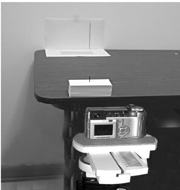
Proceeding from steps 2, 3 and 4 (**with the horizontal arm mounted to the rotator and the camera properly mounted to the camera mounting block**) now position the tripod in front of the nail and line with the camera **CAREFULLY** resting on top of the horizontal arm.
